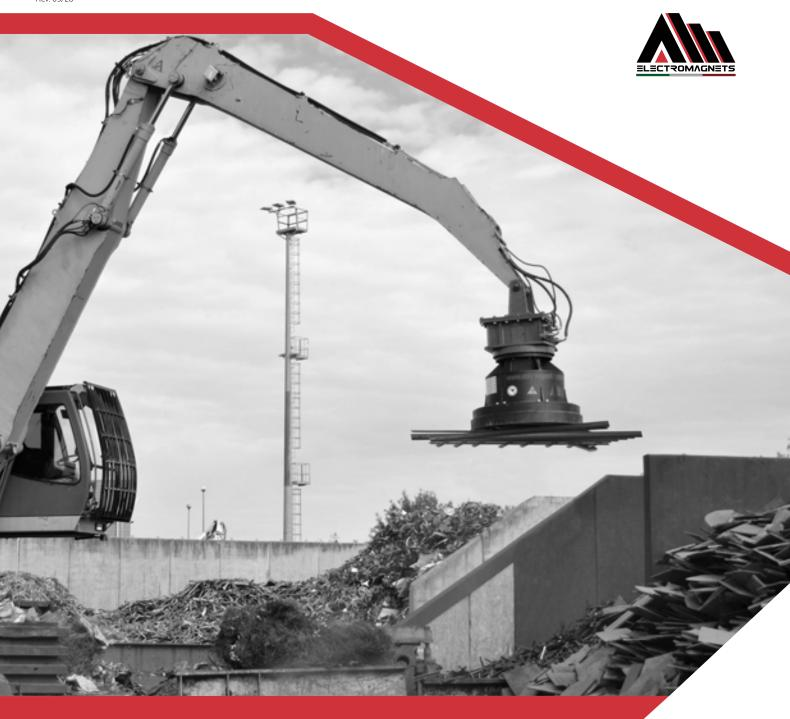
Hydraulic electromagnets with 360 deg rotation
